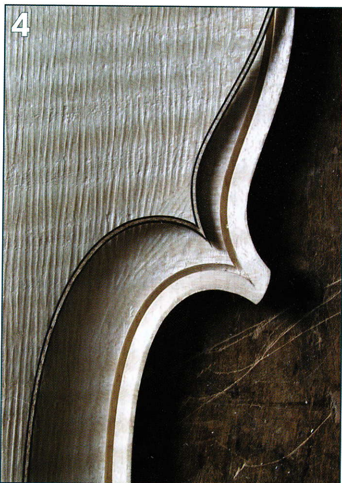
My custom-made knife is sharpened all around the blade to help cut the purfling channel
