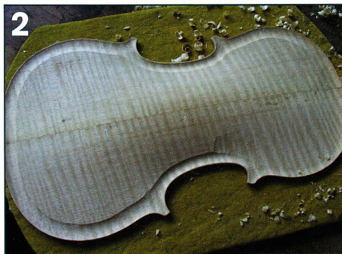
Once the channel is completed, the arching can be finished roughly
