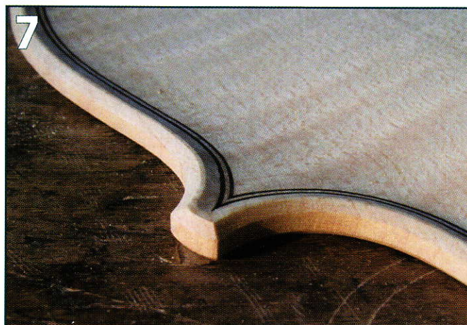
The sharp edge between the channel and the bevel needs to be softened
